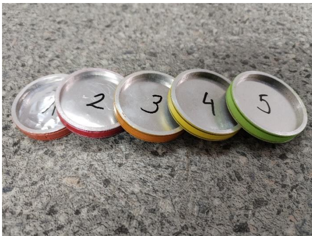
Figure 2. Aluminum beta radiation filters from 1 to 5 in radiation laboratory LARA 10
