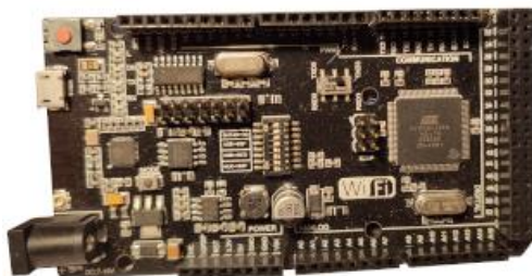
Figure 6. Arduino clone with integrated ATMEGA 2560 and ESP8266EX chip on one board
