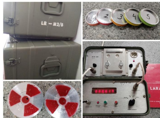
Figure 1. Parts of LR-M2 radiation laboratory: housing, filters, radioactive calibration source, scaler Svit 10 with timer
