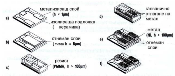
Figure 8. Sequence of a technological process for the production of a sensor
