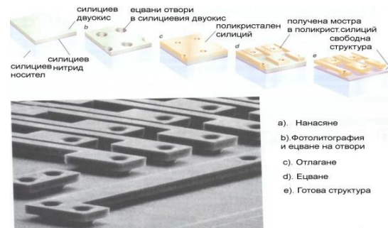
Figure 6. Technological process of acceleration sensor
